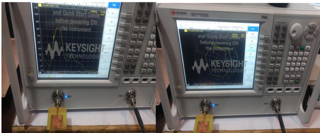
Fig. 16 Measurement set up of VSWR & input impedance at 7GHz
