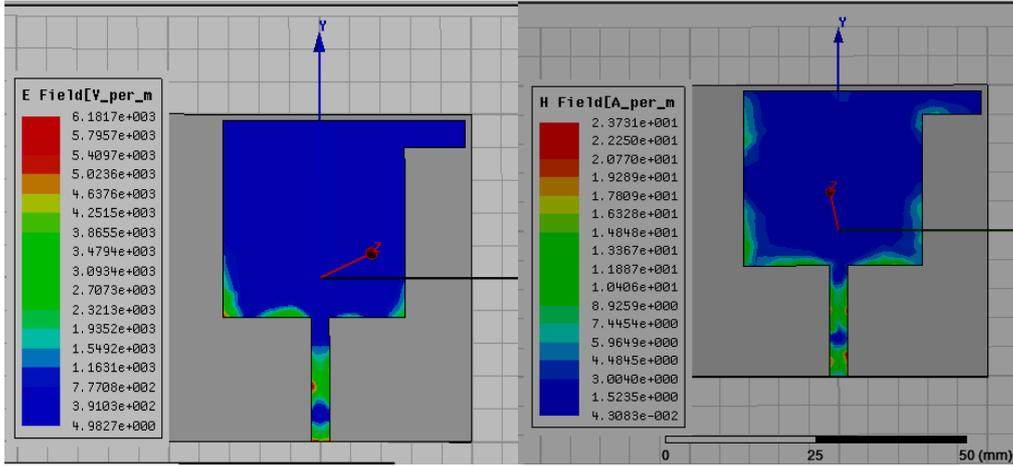
Fig. 11 E Field at 7GHz & H Field at 7GHz
