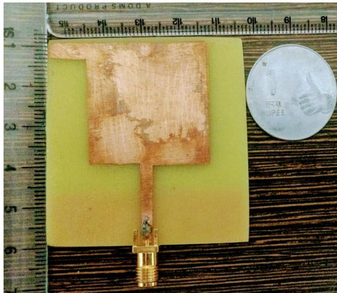
Fig. 14 Fabricated design of proposed antenna
