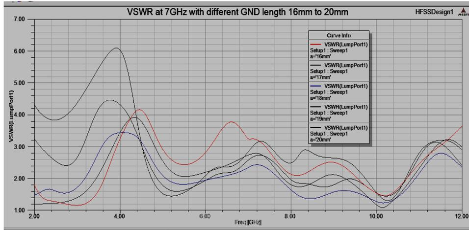
Fig. 7 VSWR of dual band patch antenna
