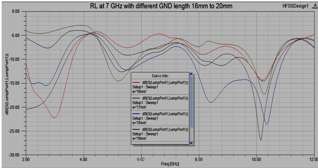
Fig. 5  $S_{11}$  of Patch antenna with different ground plane effect  $L_g$ .
