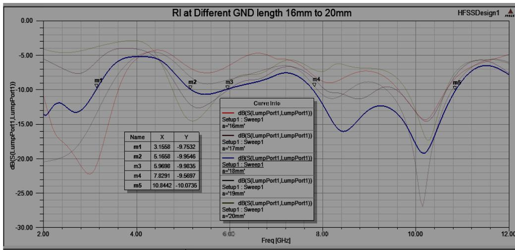
Fig. 6  $S_{11}$  of patch antenna with  $L_g=18mm$ .
