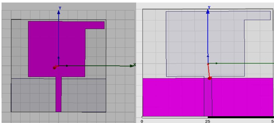
**Fig. 3** Geometry of rectangular patch Top View & Bottom View
