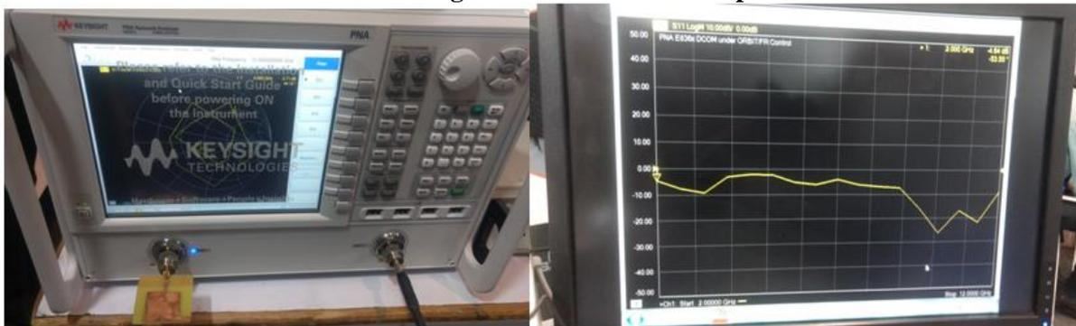
Fig. 15 Measurement set up of fabricated design & Measured Result of  $S_{11}$  at 7GHz
