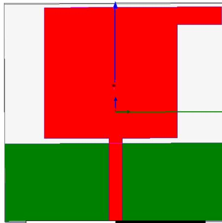
**Fig. 2** Geometry of rectangular patch
